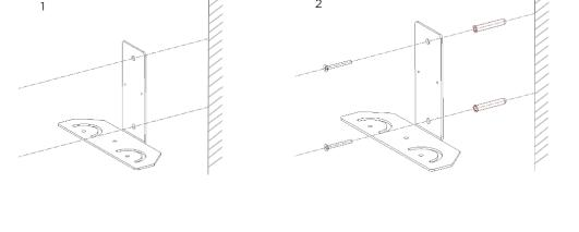
Use the bracket to mark and drill the necessary holes in the wall. \*NOTE: wall
