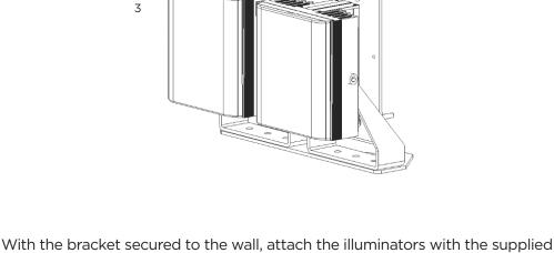
illuminator, attach the center bolt first then rotate the illuminators to the required horizontal position. Once the necessary position is achieved, secure
