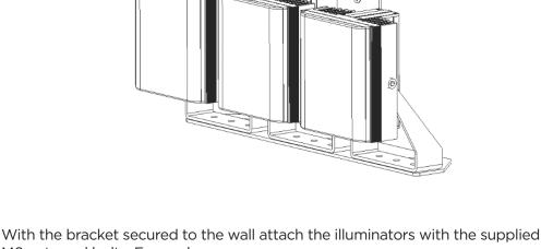
M6 nuts and bolts. For each illuminator attach the center bolt first then rotate the illuminators to the required horizontal position, then secure with the remaining nut and bold in
