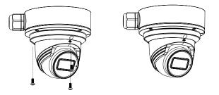
Adjust the camera's position and angle by loosening the lock screw at the base of the camera. When the camera's desired position is achieved, secure the lock screw back in place to complete the installation.
